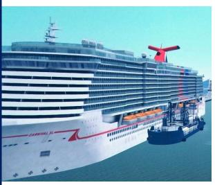
(Articulated Tug/Barge) moored alongside outboard side of Cruise Ship after Cruise Ship is safely docked and secured
